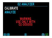
▲ DANGER: Your new DSX and O2 Analyzer cable are paired and precisely tuned at the factory, to compensate for resistance in the cable. ONLY use the cable that ships with your DSX. The cable serial number (labeled on the cable) must match the serial number that displays on your DSX (O2 Analyzer Sub Menu) screen. Contact your Apeks Dealer for assistance if the Oxygen Analyzer cable ever needs to be replaced.
